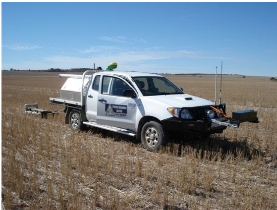
Figure 3; Gamma-ray spectrometer mounted on front of survey vehicle and EM38 towed on sled at rear.
